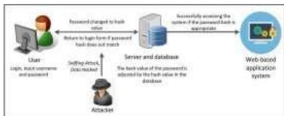
Figure 1. Working Mechanisms of One Way Hash function
