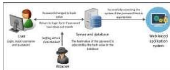
Figure 1. Working Mechanisms of One Way Hash function
